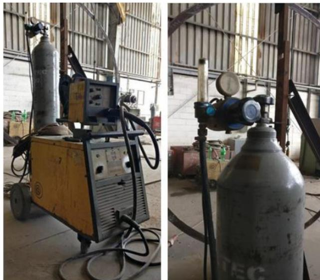
Figure 1. Gas metal arc welding (GMAW) process setup used for welding data collection
