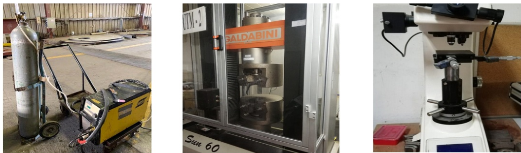
Figure 4. GTAW welding equipment, UTS and hardness machines used for experiment work
