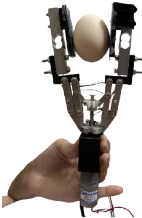
Figure 8. Fragile-object validation through grasping of a chicken egg
